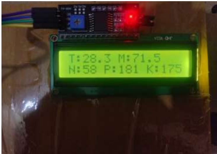
Fig. 5. LCD output showing live NPK values and recommended fertilizer.
