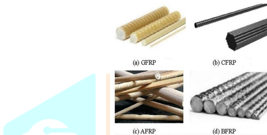
Figure 1: Four types of FRP bars [9].
