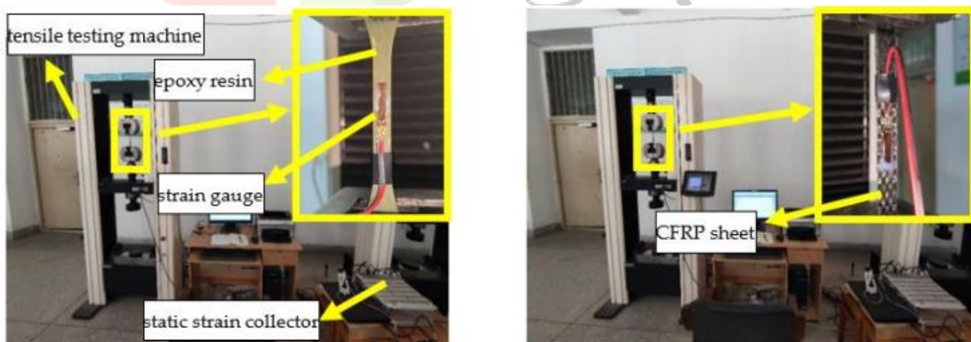
Figure 9: Stress testing of epoxy resin and CFRP
